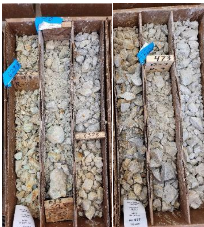
Figure 12.3: YM-047A and YM-049 Footage Blocks and Tags
