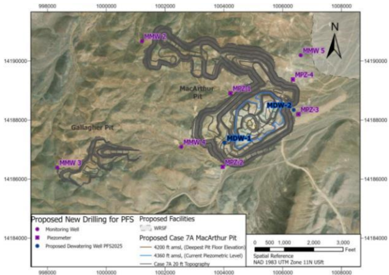
Figure 18.3: Potential Location for MacArthur Pit Dewatering and Monitoring Wells
