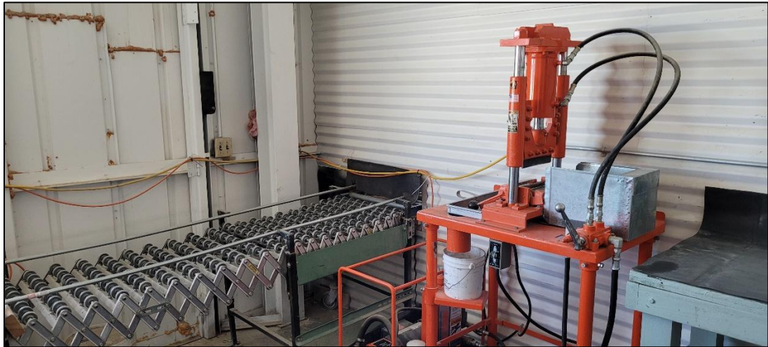
Figure 11-2: Splitter in Sample Room Connected by Conveyor with Core Logging Facility
